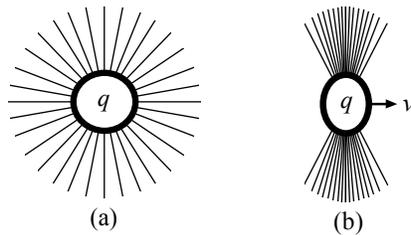
**Figure 2.** Electric Field Intensity of Charged Sphere, from equation (IV). Part (a) shows the field lines for the charge at rest. Part (b) shows the field lines for the same charge moving at a velocity  $0.94c$ , so that  $\beta = 0.94$ .
